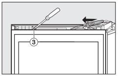
Screw the spacer and the soft-close mechanism together securely using screw (3).
